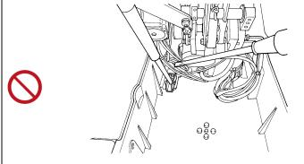
Whenever you find that the gas spring does not move or function normally, replace the gas spring with a new one.
