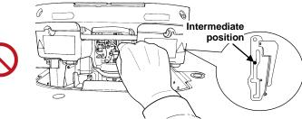
Be sure to lift up the sewing machine until the hinge stopper is locked at the threading position to secure the sewing machine.
