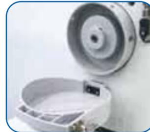
The handwheel cover prevents the sewing machine from starting up unexpectedly while the operator is turning the handwheel by hand. In addition, the cover also prevents the thread and material from being entangled in the handwheel during sewing.
