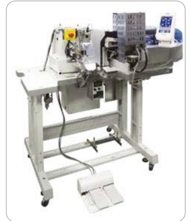
The AB-1360 / CR-10A sewing machine with a preset loader automatically feeds shoelace loops and shoe tongues to the correct shoelace loop attaching position, thereby no longer requiring manual positioning of those parts. The sewing machine is an automatic machine which realizes full-automatic sewing while eliminating inconsistency in quality and sewing position faults caused by the operator.
