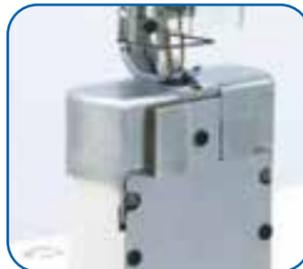
The sewing machine will not start if the throat plate is open. This prevents the material from being caught in the hook during sewing.
