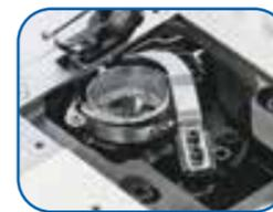
The thread trimming mechanism has been completely renewed. The industry's shortest remaining thread length achieved by trimming the thread close to the fixed knife at the last stitch (condensed stitch). The length of remaining needle thread is 5mm.
