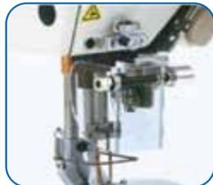
The eye guard prevents a broken needle from flying off. If the eye guard is open, the sewing machine cannot be started. As a result, the sewing machine will not start up unexpectedly even if the operator forgets to turn the power off.
