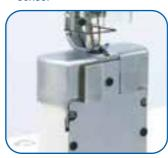
The sewing machine will not start if the throat plate is open. This prevents the material from being caught in the hook during sewing.
