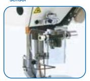
The eye guard prevents a broken needle from flying off. If the eye guard is open, the sewing machine cannot be started. As a result, the sewing machine will not start up unexpectedly even if the operator forgets to turn the power off.
