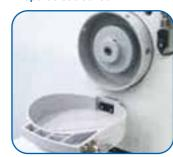
The handwheel cover prevents the sewing machine from starting up unexpectedly while the operator is turning the handwheel by hand. In addition, the cover also prevents the thread and material from being entangled in the handwheel during sewing.
