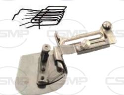
Stitched elastic swing out hemmer. Amount of gathering is obtained by adjusting a special tension bracket. This is an upturn hemmer that stitches in elastic end to end while sewing.
