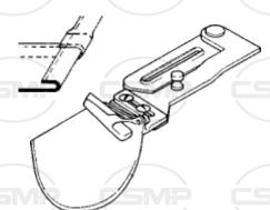
Single upturn spring hemmer complete on swing bracket. Designed for hemming through seams. Made in Italy by CF Italia.
