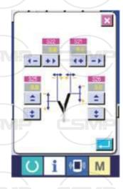
The cutting of the corner-knife can be adjustment through the operation panel
