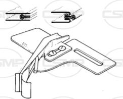
Cord edge piping attachment with foot made by CF Italia.
