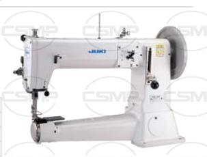
**JUKI LK-1942HA** (For Heavy-Weight with Intermediate Presser) **JUKI LK-1942GA** (For Extra Heavy-Weight with Intermediate Presser)
