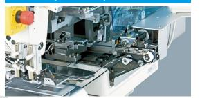
The belt-loop feeder unit incorporates JUKI's unique twin system. It is able to feed belt-loops with consistency even when a soft and elastic material is used. The belt-loop feeder unit is arranged in front of the main body of the sewing machine. This allows the operator to insert belt-loops from the front of the machine. In addition, the operator can visually check the belt-loop state whenever necessary, even during sewing.
