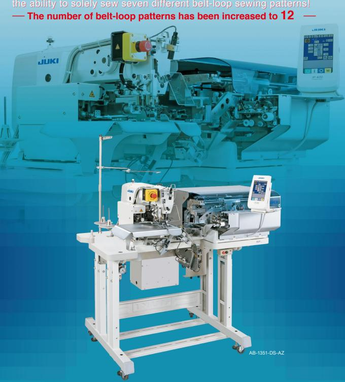
**Automatic 1-needle Belt-Loop Attaching Machine**
