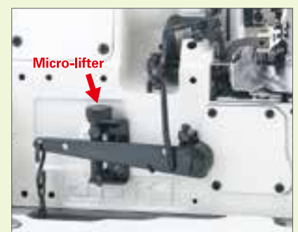
Bottom and top differential-feed micro adjustment mechanism
