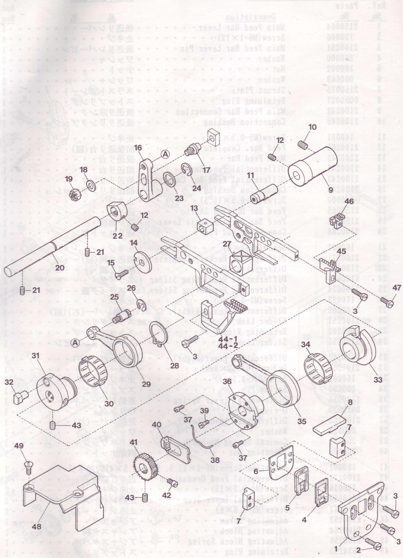
FEED DRIVING MECHANISM
