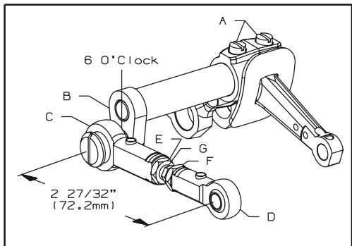
At this time the knife drive lever should be in the 6 o'clock position. If adjustment is necessary, loosen screws (A, Fig. 28) in the needle lever and reposition knife drive lever (B) to the 6 o'clock position. Tighten screws (A). The dimension between the centerline of right and left knife drive connection ball joints (C and D) must be 2 27/32" (72.2mm). Loosen left hand thread nut (E), right hand thread nut (F) and turn connecting rod (G) until dimension is achieved. Tighten nuts (E and F).
