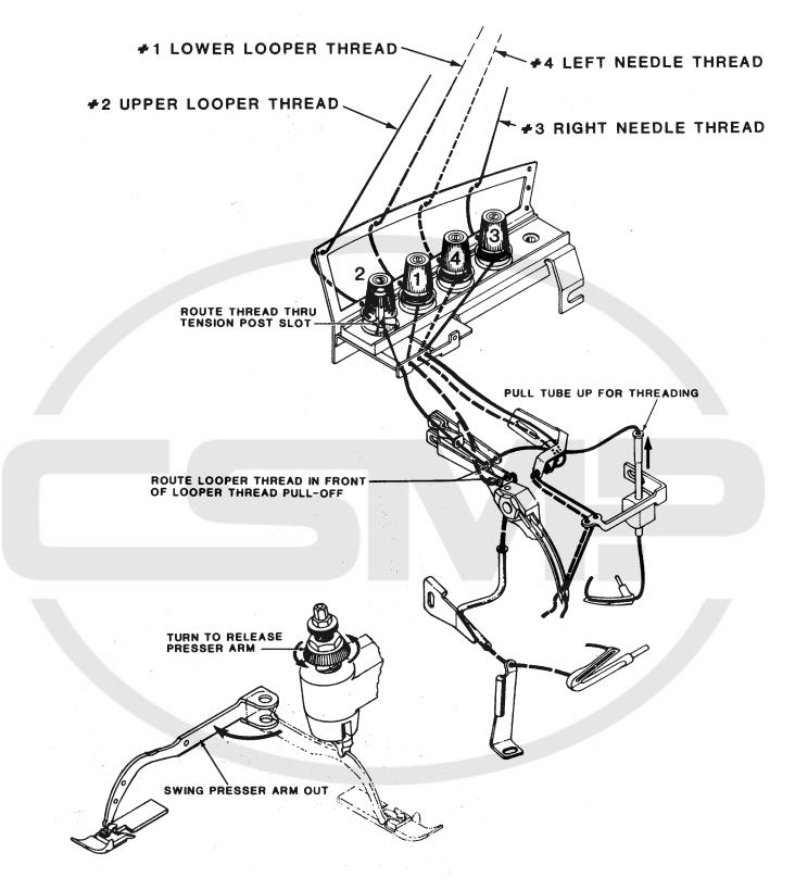
Thread machine in sequence as shown: (1) lower looper thread, (2) upper looper thread, (3) right needle thread and (4) left needle thread.
