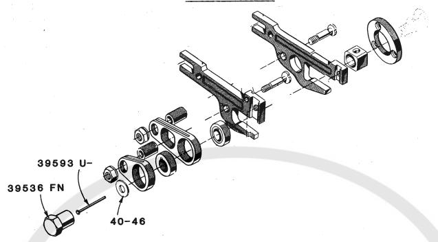
Beginning with machine serial number 1620485 the wood oil metering plug is now being replaced by a steel metering pin which is inserted inside the main shaft on all Class 39500 Machines.
