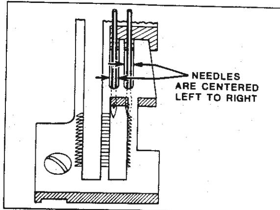
If adjustment is required, remove fabric guard and looper thread pull-off. Loosen needle driving arm clamp screw (A, Fig. 6) and reposition arm to the right or left as necessary. Temporarily tighten clamp screw, (A), then proceed to check needle(s) height.
