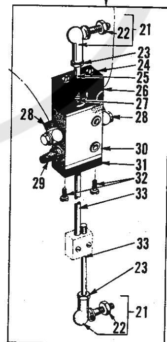
VENTURI TUBE, PNEUMATIC CONTROL DEVICE, TREADLE ROD VALVE
