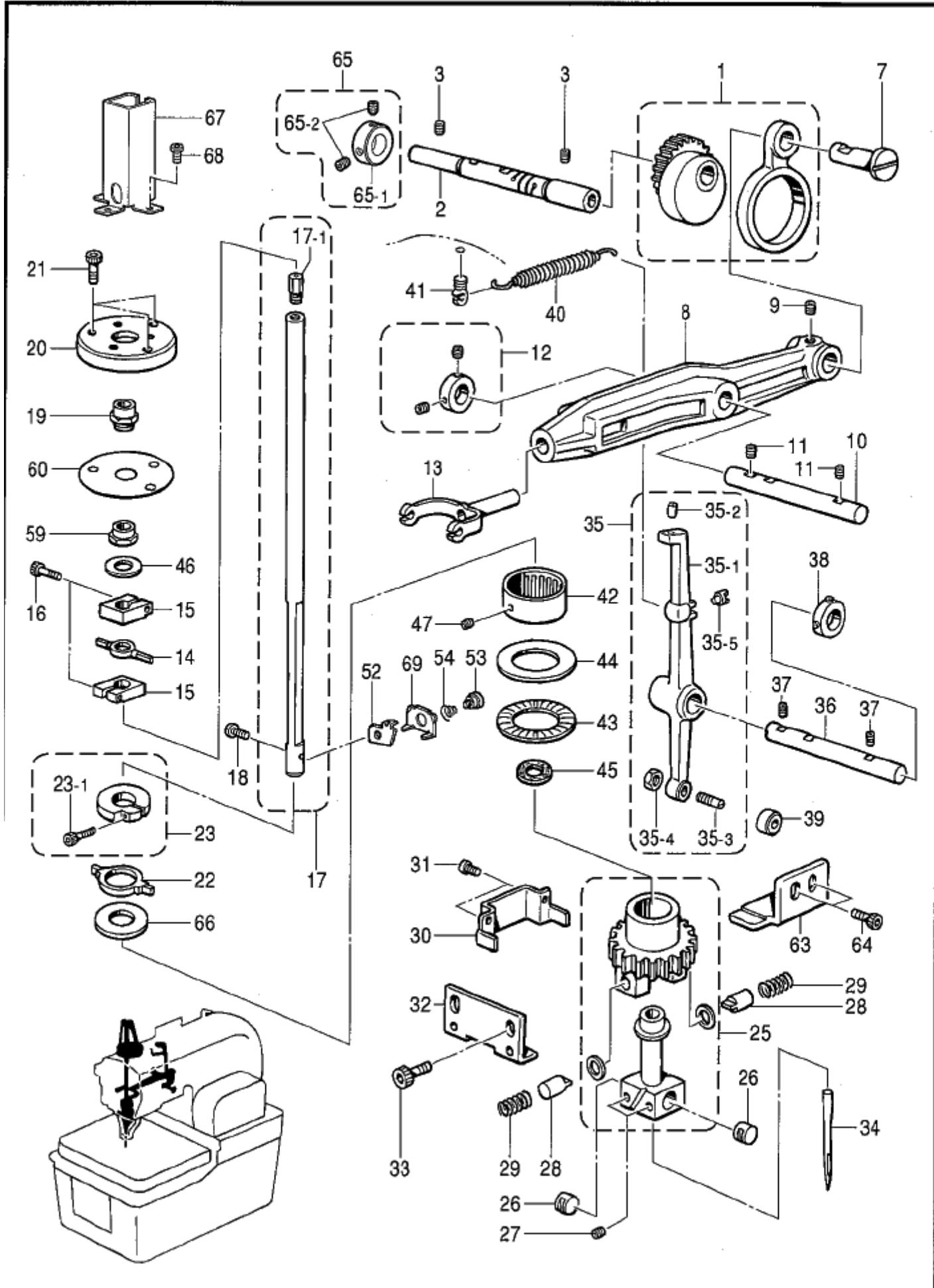
B . 針棒・天秤関係 / Needle bar and thread take-up mechanism
