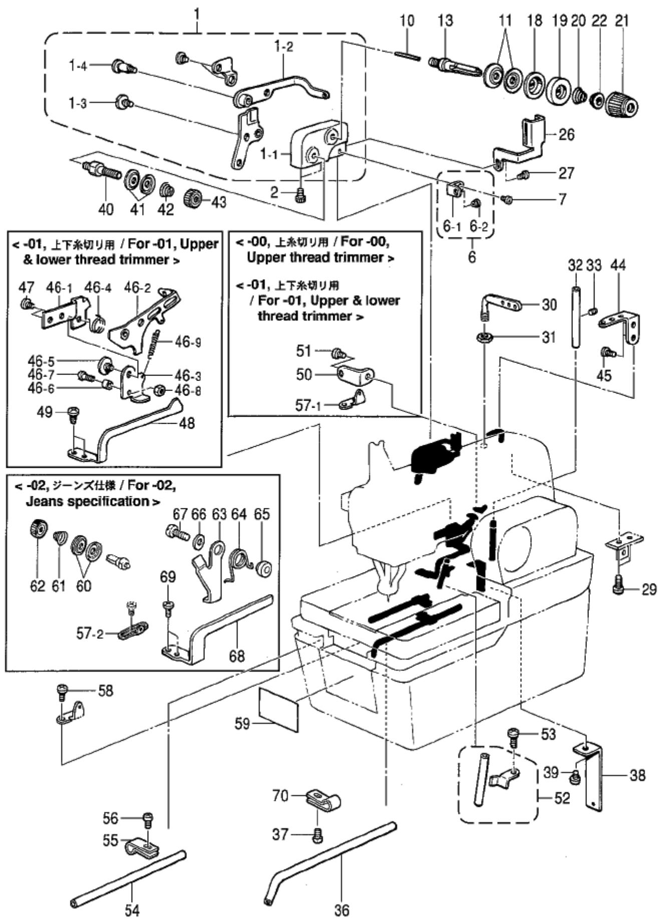
Q. 糸通し関係 / Threading mechanism
