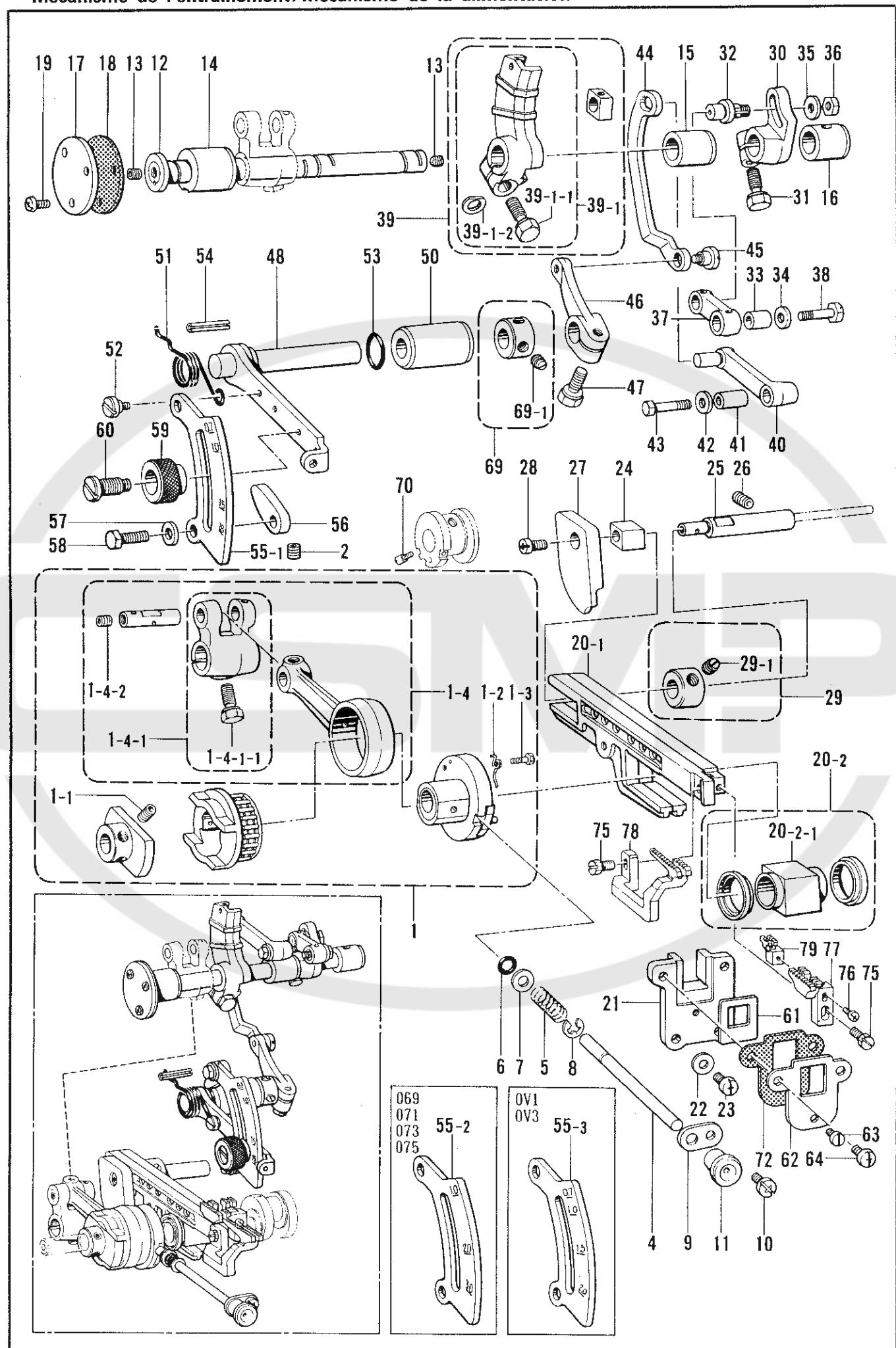
F. 送り関係/Feed mechanism/Transportvorrichtung/
