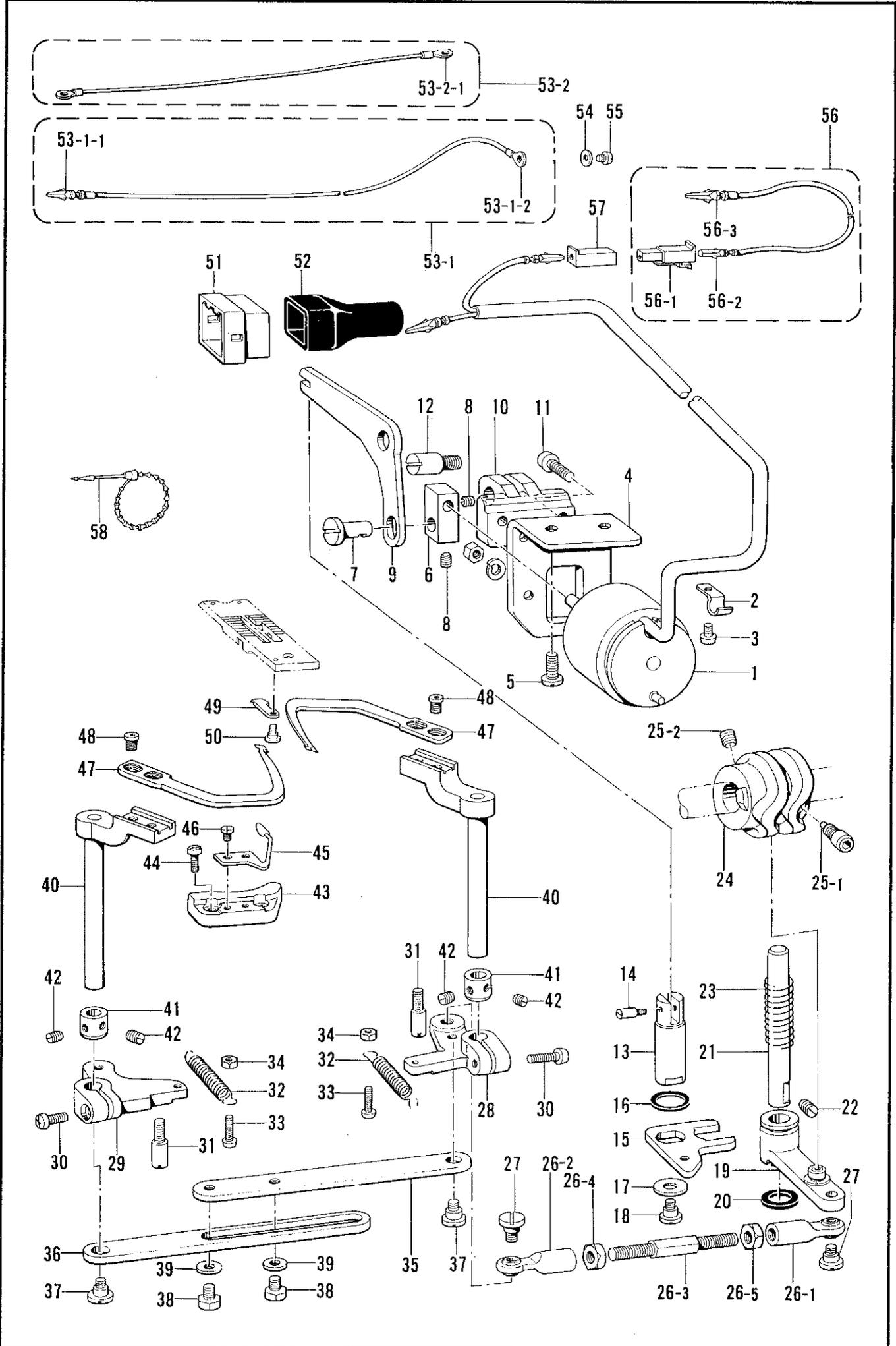
N. 糸切り関係 (糸切り)/Thread trimmer mechanism (Thread Trimmer)/
