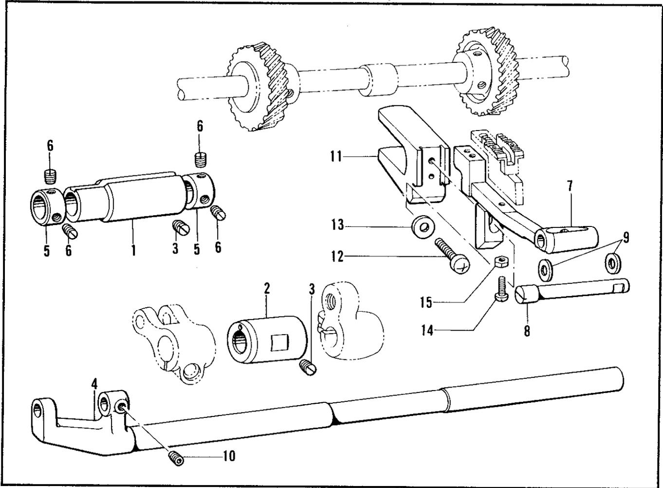
G1. 押工上げ関係 / Work clamp lifter mechanism /
