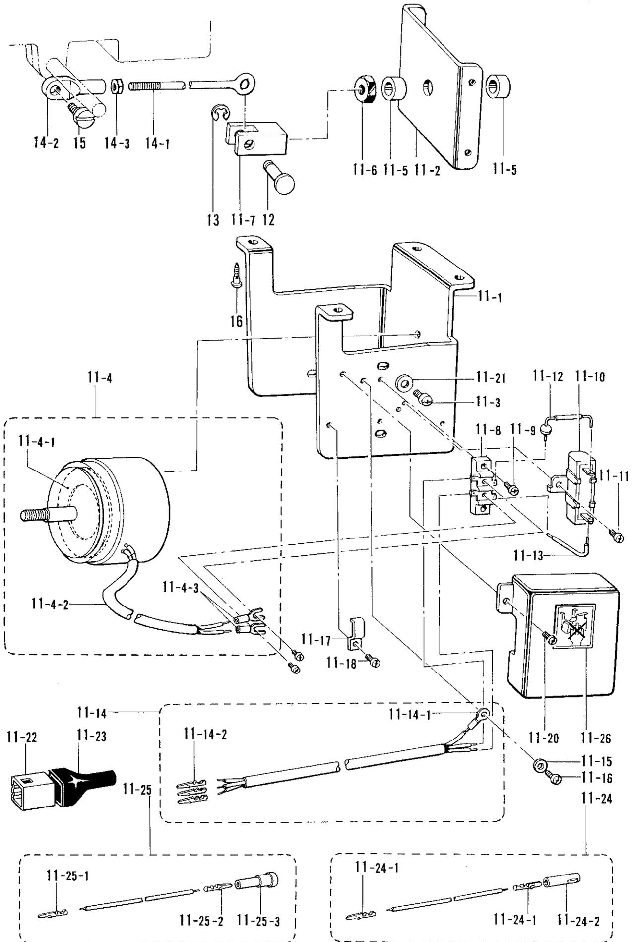
G2. 押工上げ関係/Work clamp lifter mechanism/
