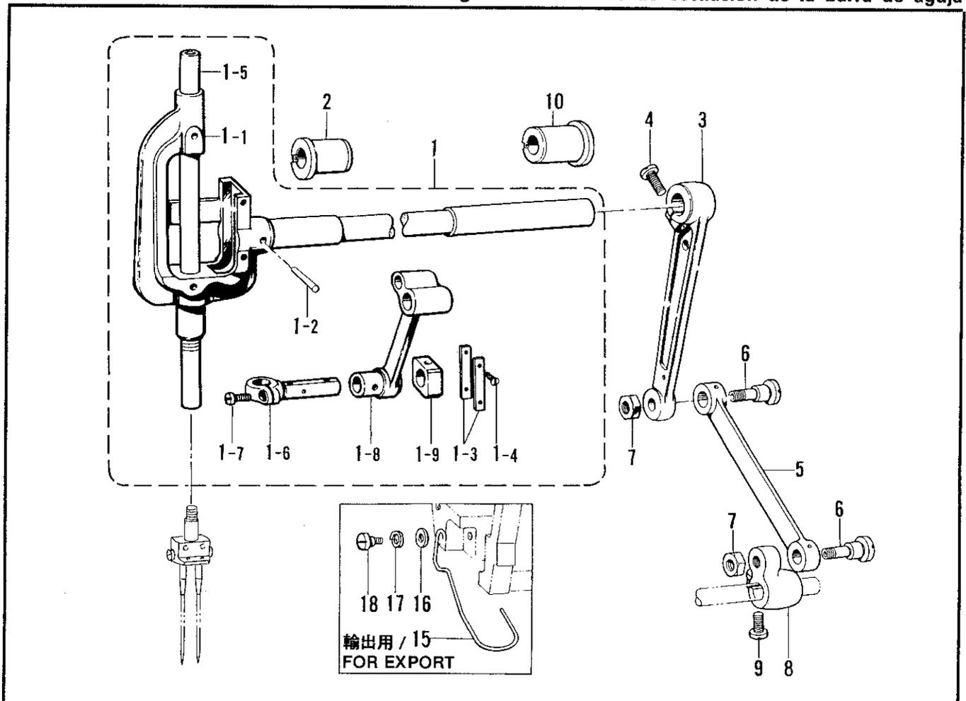
B. 上軸関係/Upper shaft mechanism/Obere Welle/
