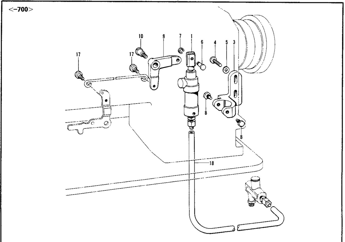
F. 送り軸関係/Feed shaft mechanism/Transport welle/
