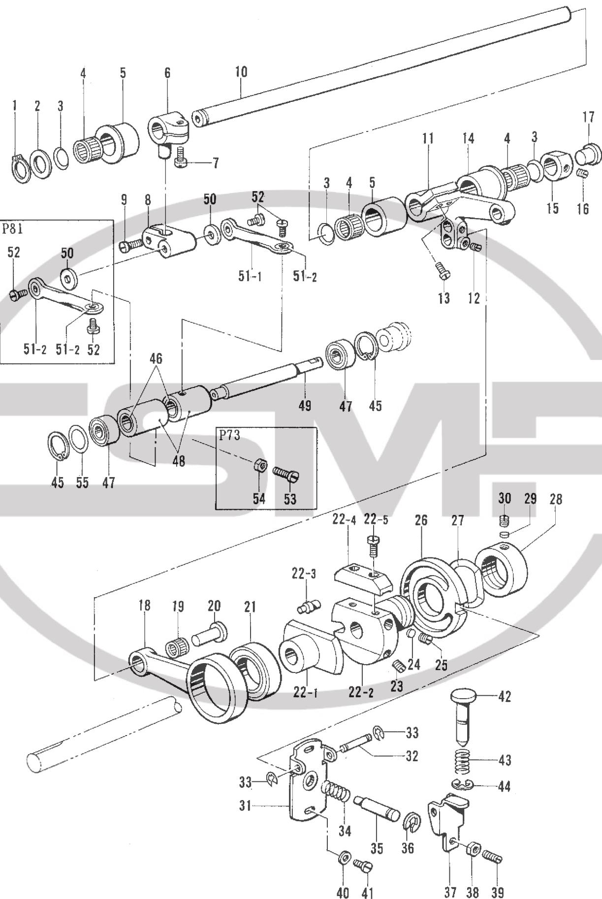
D. 送り関係/Feed mechanism/Transportvorrichtung/
