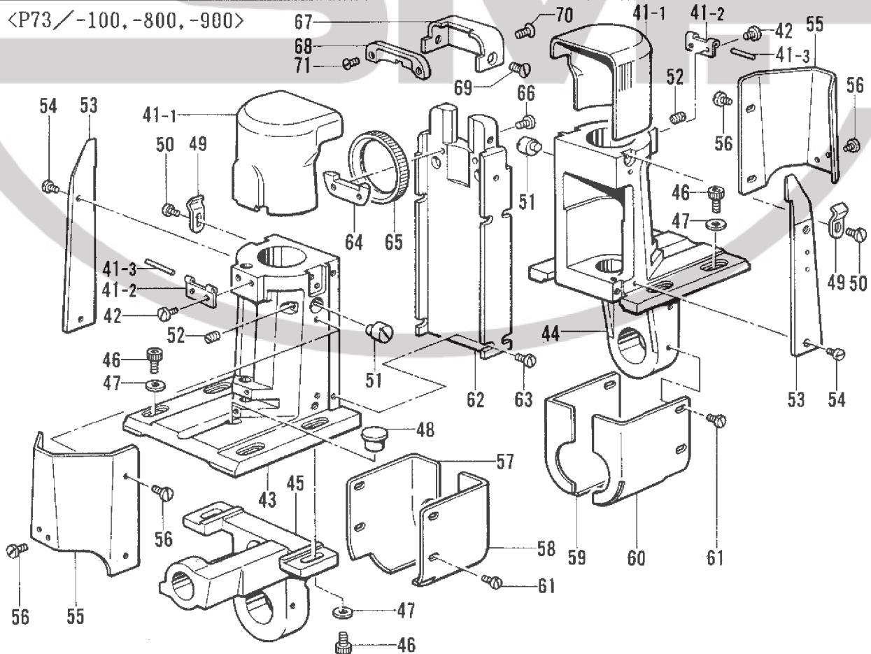
J5. カマ関係/Rotary hook mechanism/Greifervorrichtung/
