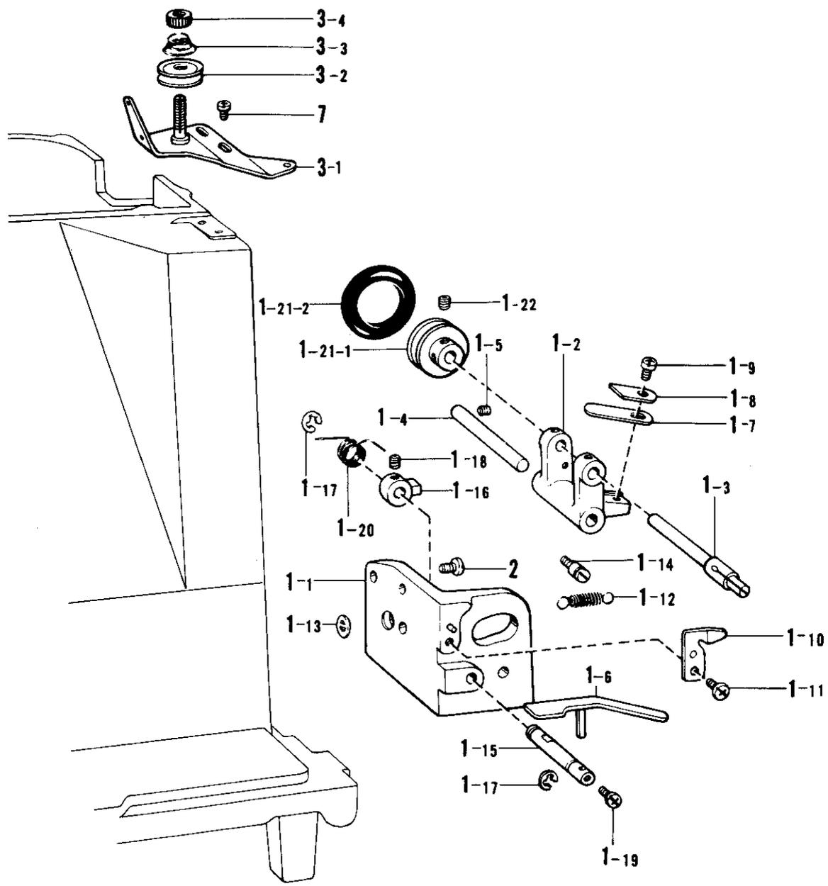
M. 糸巻キ関係/Bobbin winder mechanism/Spuler
