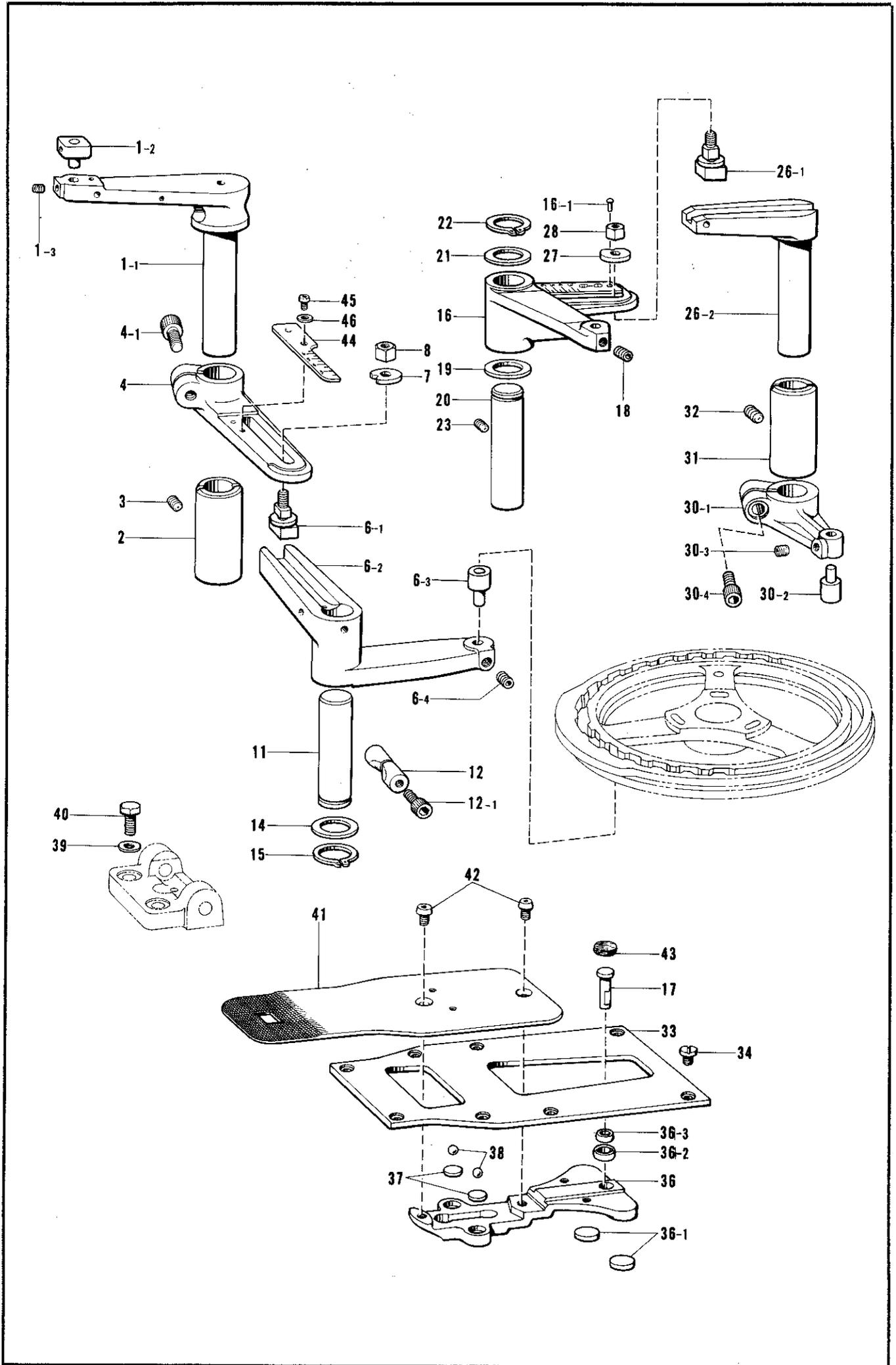
E. 送り関係/Feed mechanism/Transportvorrichtung/
