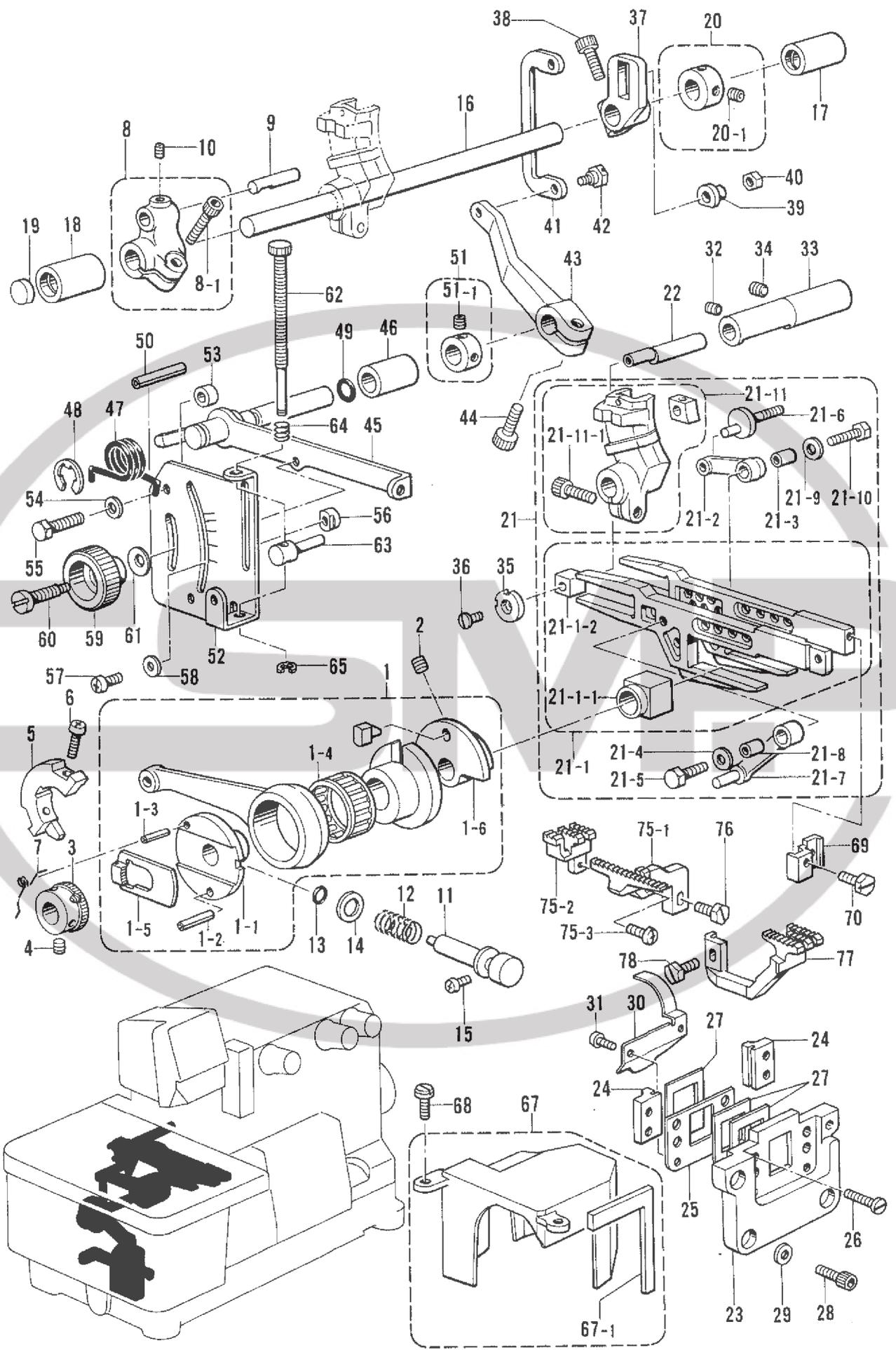
E. 送り関係/Feed mechanism/Transportvorrichtung/
