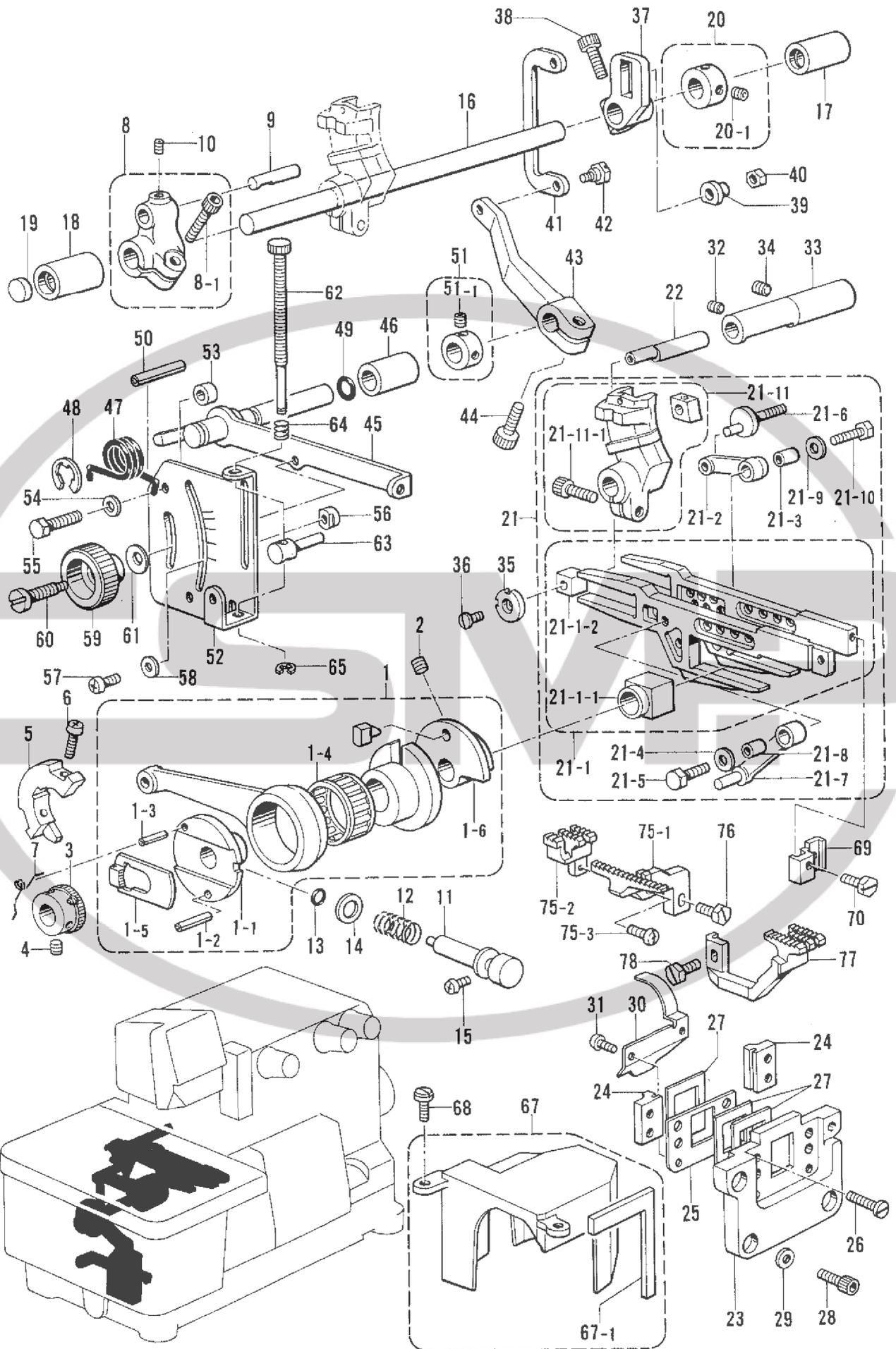
E. 送り関係/Feed mechanism/Transportvorrichtung/
