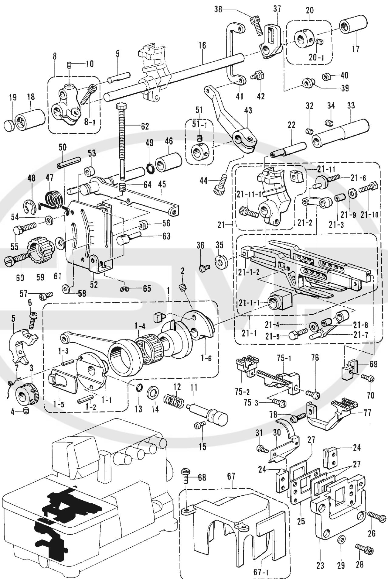
E. 送り関係/Feed mechanism/Transportvorrichtung/
