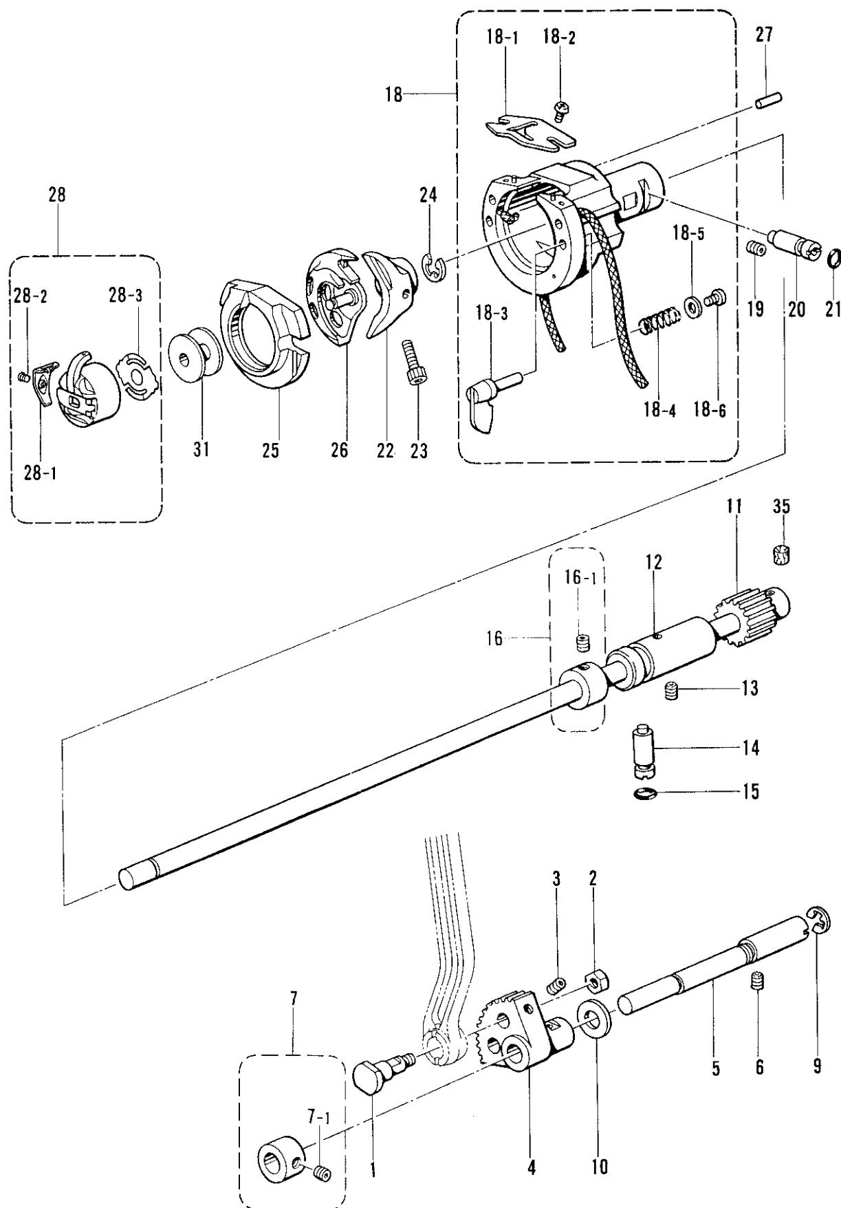
Lower shaft mechanism / Untere Welle /
